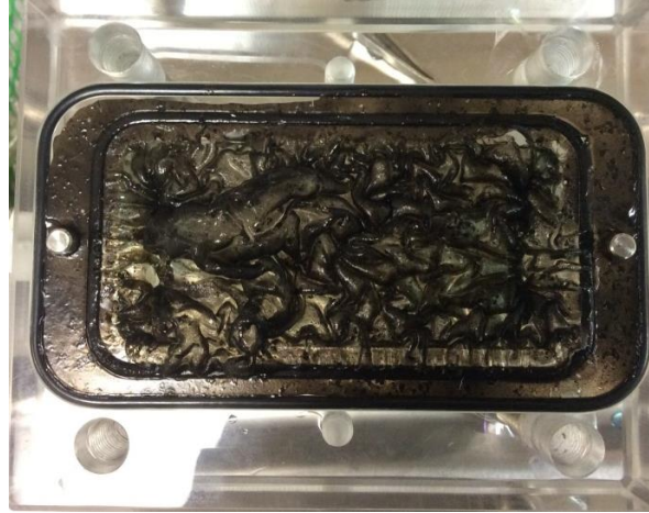
Figure 5.6 Top View of d-CSGO Membrane After Failure
