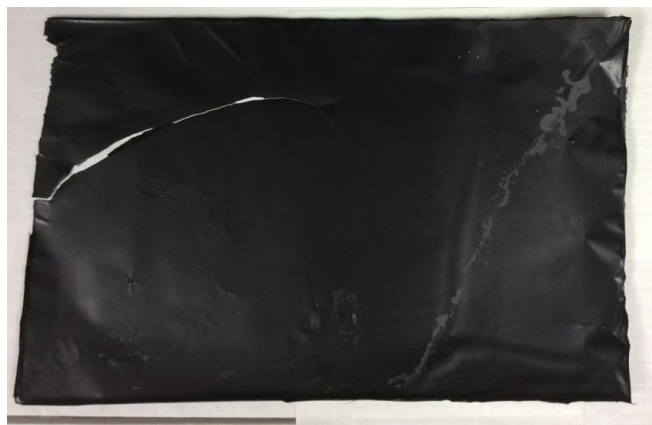
Figure 5.25 Scaled d-g-CSGO Membrane
