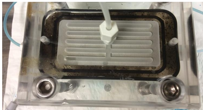
Figure 5.5 Membrane Filtering Methylene Blue (10 mg/000
