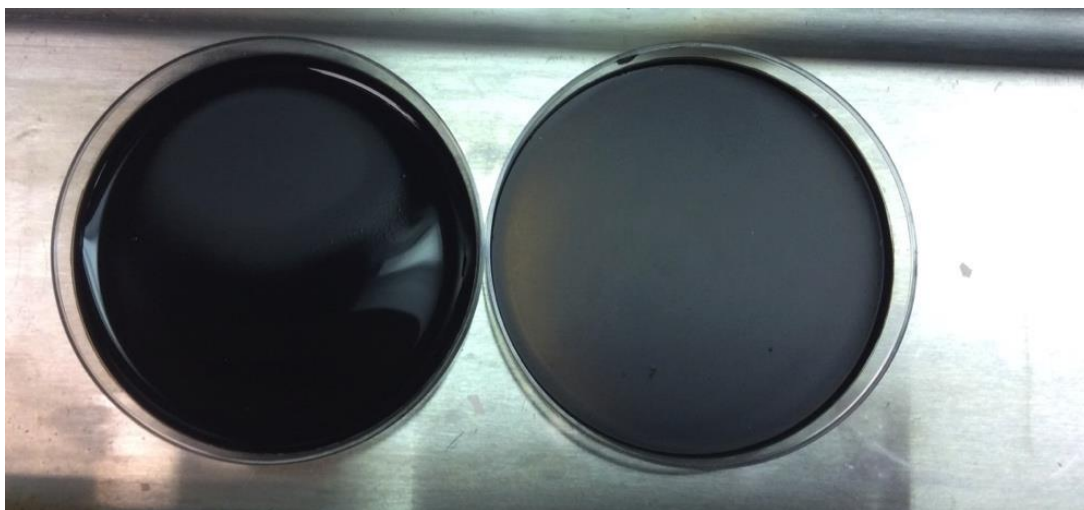
Figure 5.1 CSGO Solution After Drying for 24 Hours (Left – CSGO Solution Dried in a Bell Jar; Right - CSGO Solution Dried in an Incubator)
