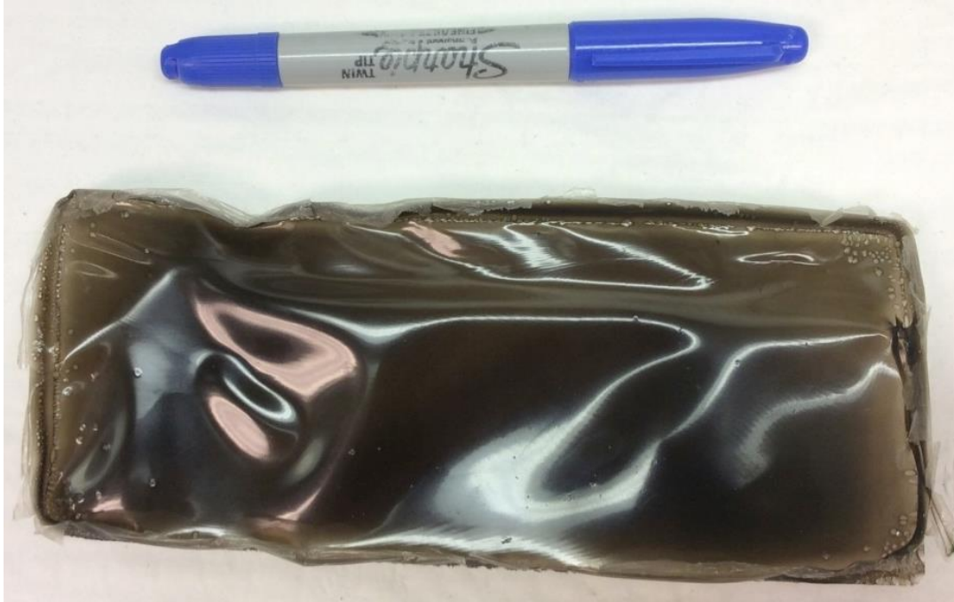
Figure 5.3 Dried d-CSGO Membrane After 72 Hours of Incubation
