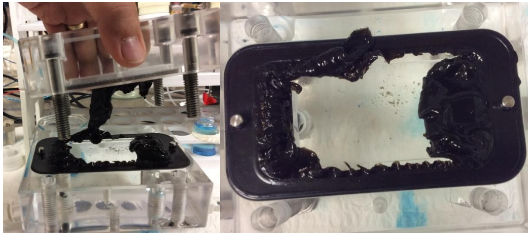
Figure 5.9 n-CSGO Membrane Failure After 6 Hours in a Cross-flow Reactor
